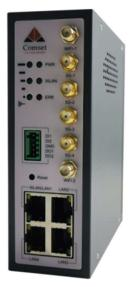
The CM550W-POE comes with three Gigabit LAN ports for fast wired connections, and one Gigabit LAN/WAN port for fixed internet, allowing for failover between 4G/5G and NBN/ADSL. It also features a GPIO with two digital input ports and two digital output ports, as well as RS232 and RS485 serial ports. Other features include VPN IPsec, PPTP, L2TP, and OpenVPN to establish a secure connection over the 4G and 5G network.
